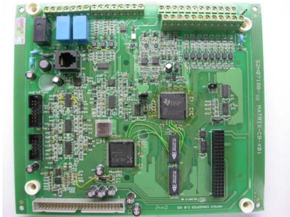
Figure 7. The photograph of the control board.
