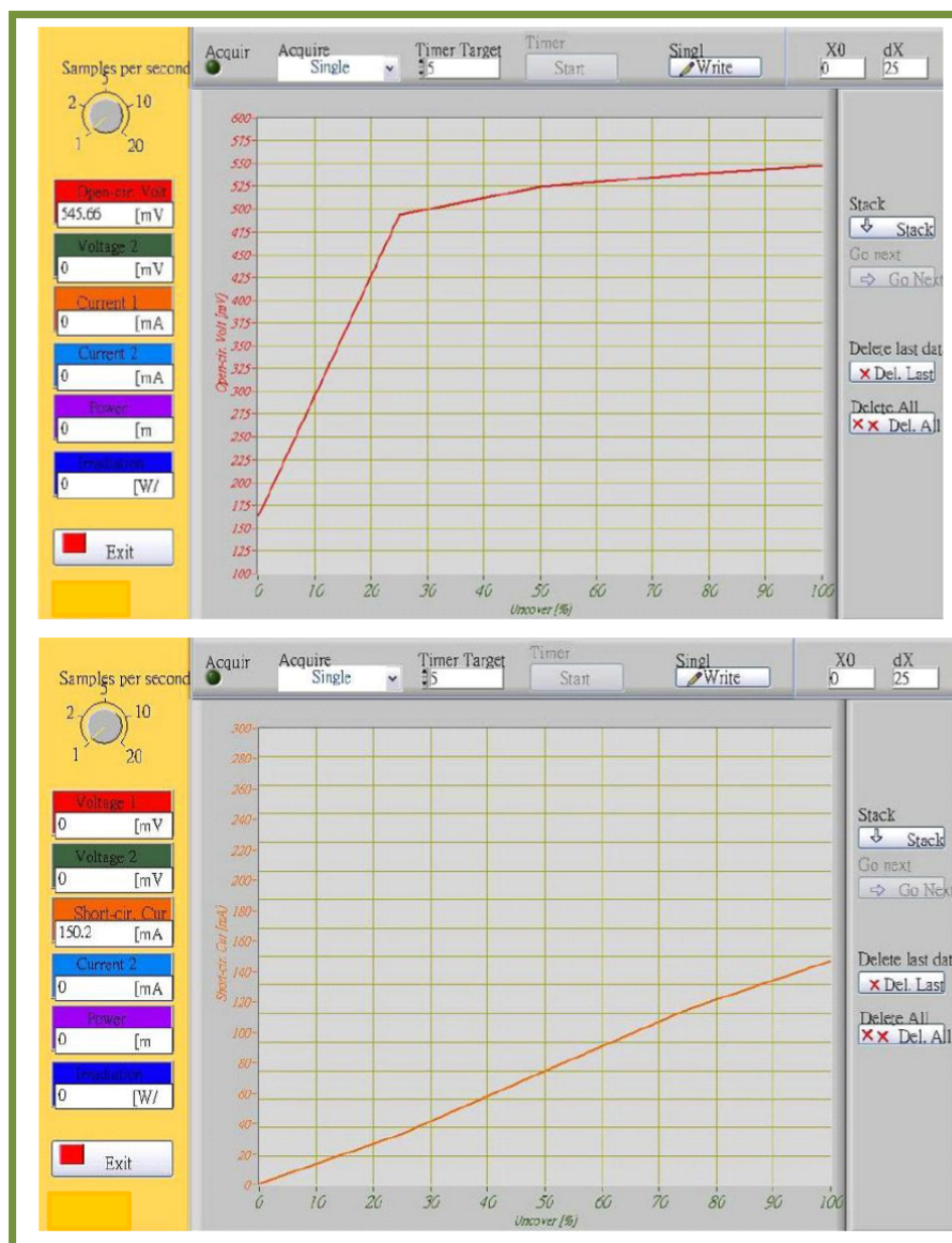
FIGURE 7. Effect of shading on open-circuit voltage/short-circuit current of PV cells
