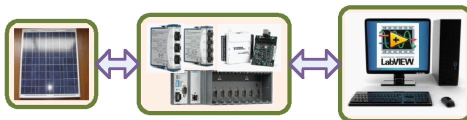
FIGURE 3. Schematic diagram of developed PV cell virtual instrumental system
