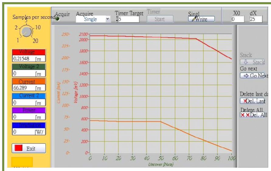
FIGURE 5. I-V and voltage/current-irradiation curves
