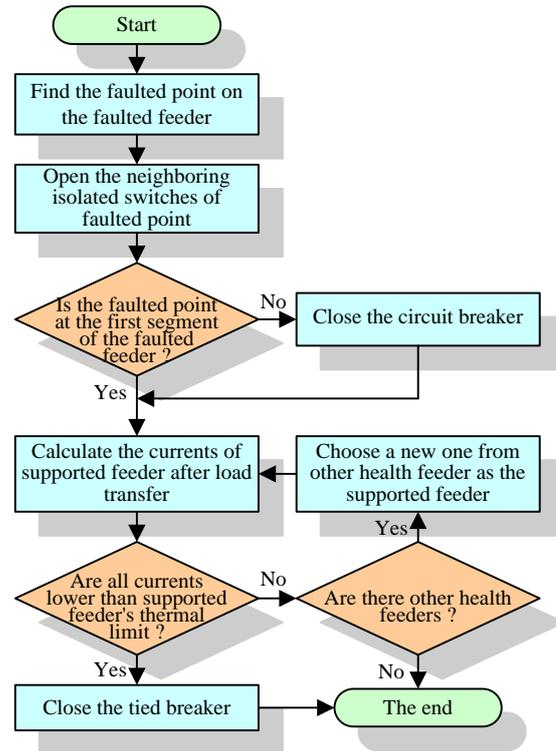
Fig. 2 Flowchart of conventional load transfer scheme
