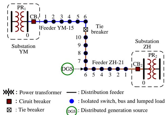
Fig. 4 The configuration of example system I
