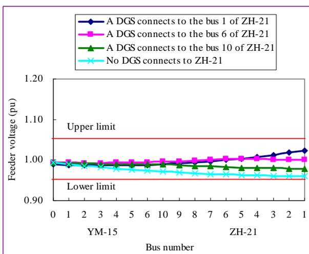
Fig.7 Voltage profiles of example feeders YM-15 and ZH-21 (DGS's power factor is 1.0)
