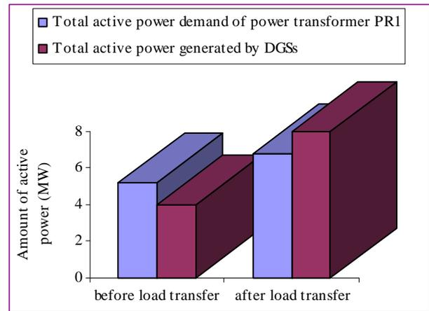
Fig. 14 The active power demand of power transformer PR<sub>1</sub> and generated by DGSs before and after load transfer
