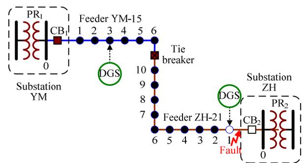
Fig.9 The connecting locations of the two DGS for the simulation scenario in subsection 4.3
