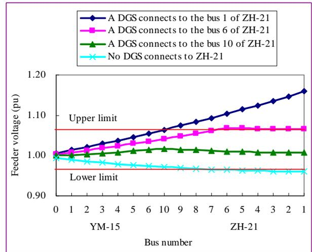
Fig.8 Voltage profiles of example feeders YM-15 and ZH-21 (DGS's power factor is 0.85 lagging)
