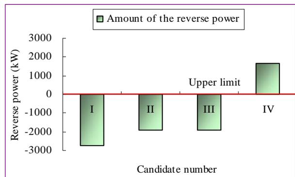
Fig.19 Reverse power of each load transfer candidate
