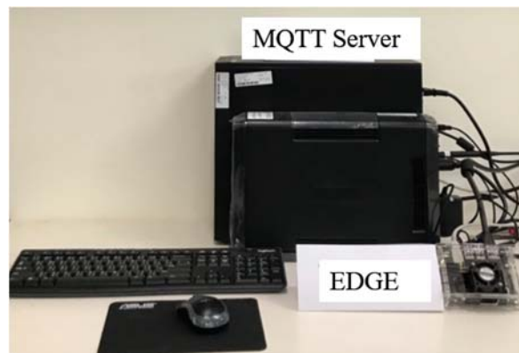
Figure 13. Prototype EDGE platform and private MQTT server.
